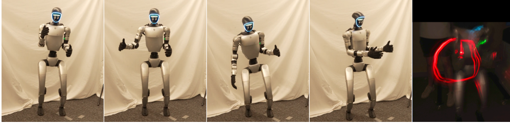
Figure 12: Impedance position control. Combining a precise force control policy with a proprioceptive state estimator, we develop an impedance controller for closed-loop end-effector position tracking. The controller tracks a circular trajectory reasonably well without any external sensing.
